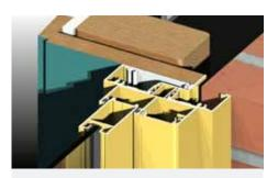
Most AWS Commercial products can incorporate nailing fins for residential construction.
